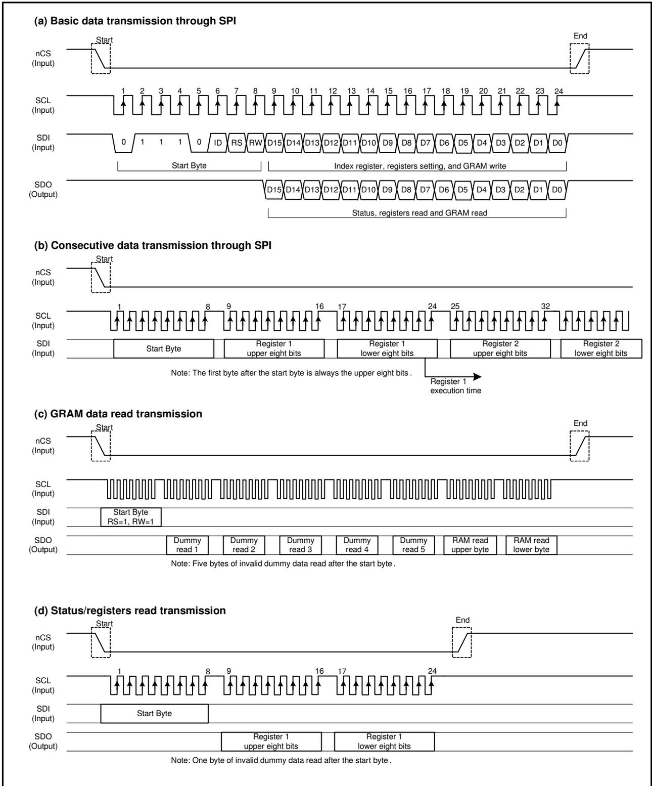
**Figure7 Data transmission through serial peripheral interface (SPI)**
