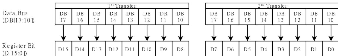
**Figure22 Register setting with i80 System Interface**
