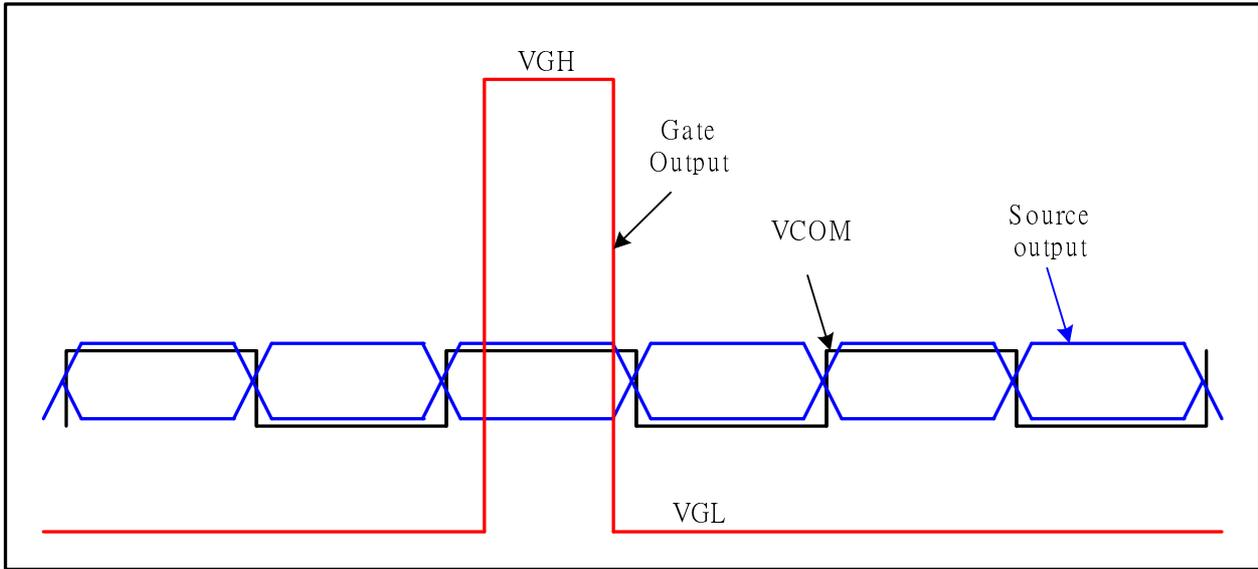
Figure 46 Voltage Output to TFT LCD Panel
