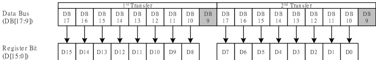
i80/M68 system 8-bit data bus interface/Serial peripheral interface (2/3 transmission)
