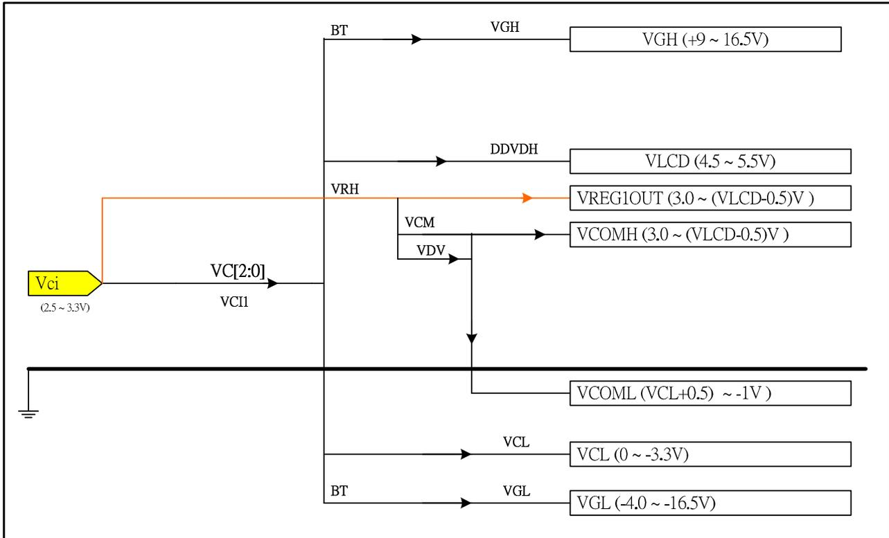
**Figure 45 Voltage Configuration Diagram**
