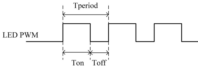
The period  $T_{period}$  of PWM pulse can be changed by the PWM\_DIV[7:0] bits of the command “PWM\_DIV (F2h)”. The LED-on time  $T_{on}$  and the LED-off time  $T_{off}$  are decided by the backlight brightness level which is calculated with CABC in ILI9325C. If CABC is off, then LEDPWM will forced to “H” level.
