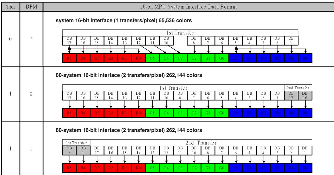
**Figure25 16-bit MPU System Interface Data Format**
