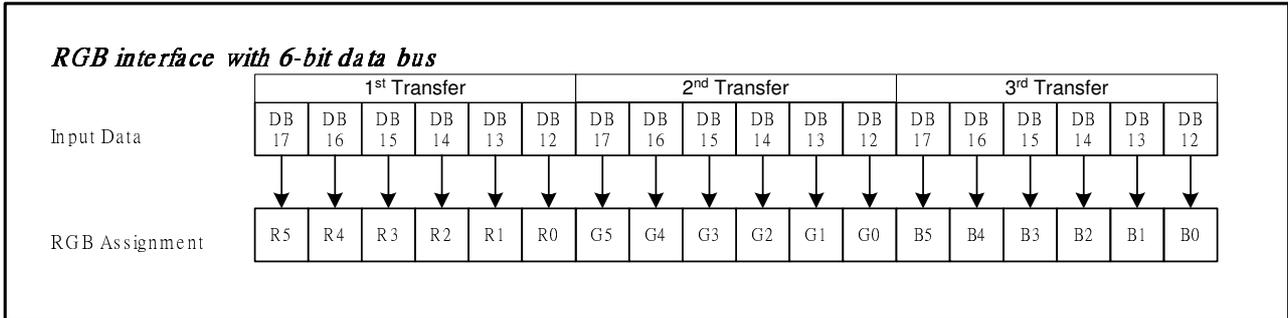
**Data transfer synchronization in 6-bit RGB interface mode**
