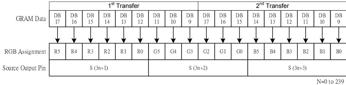
GRAM Data and display data of 18-/16-/9-bit system interface (SS=" 0", BGR=" 0")
