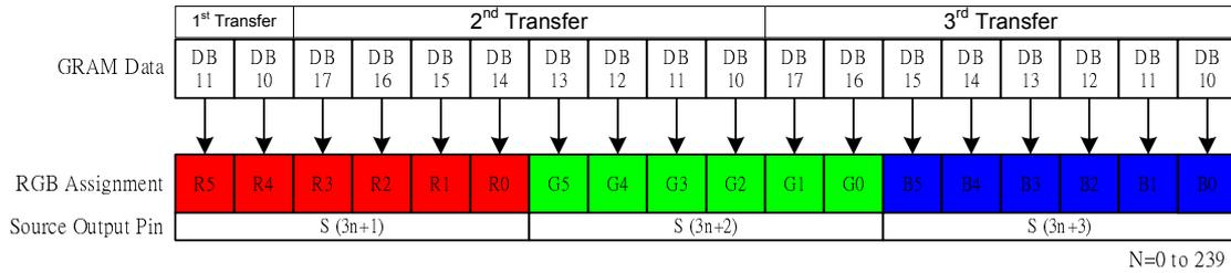
*i80M68 system 8-bit interface (3 transfers/pixel, TRI=" 1", DFM[1:0]=" 10)*
