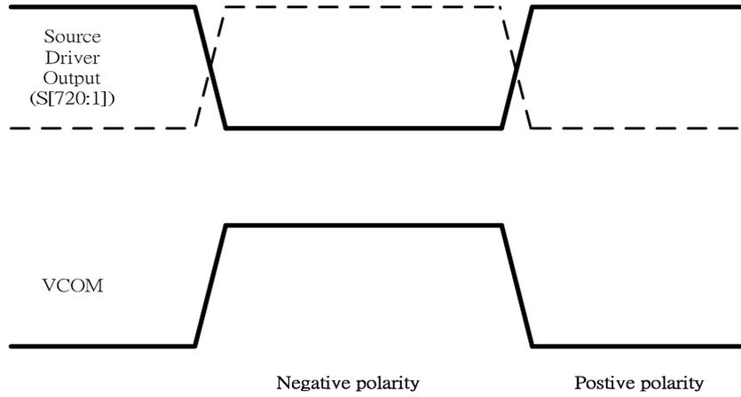
**Figure 39 Relationship between Source Output and VCOM**
