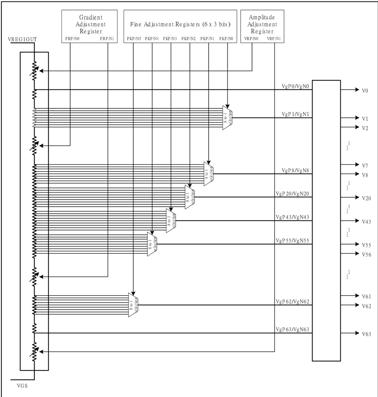
Figure 35 Grayscale Voltage Generation
