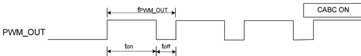
Note : The output frequency tolerance of internal frequency divider in CABC is ±10%
