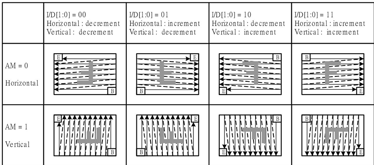
**Figure24 GRAM Access Direction Setting**
