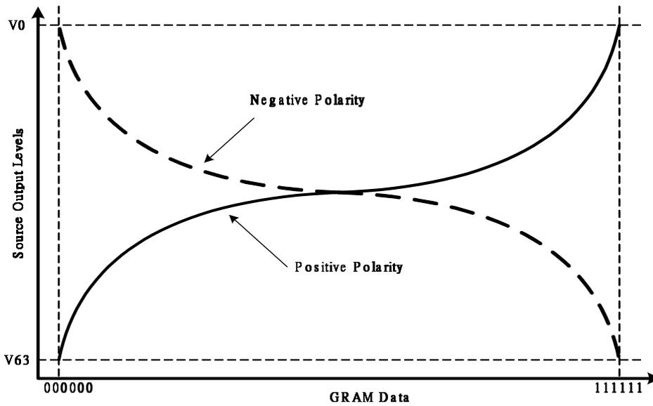
**Figure 40 Relationship between GRAM Data and Output Level**
