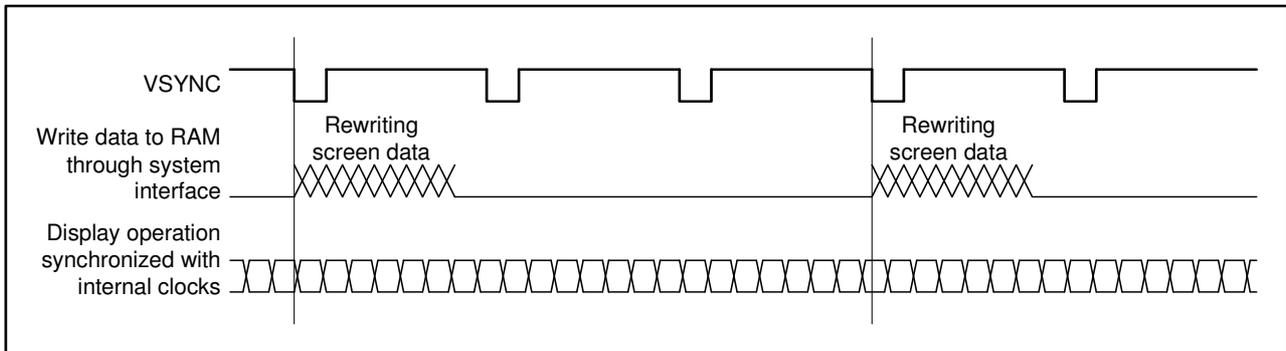
**Figure10 Moving picture data transmission through VSYNC interface**
