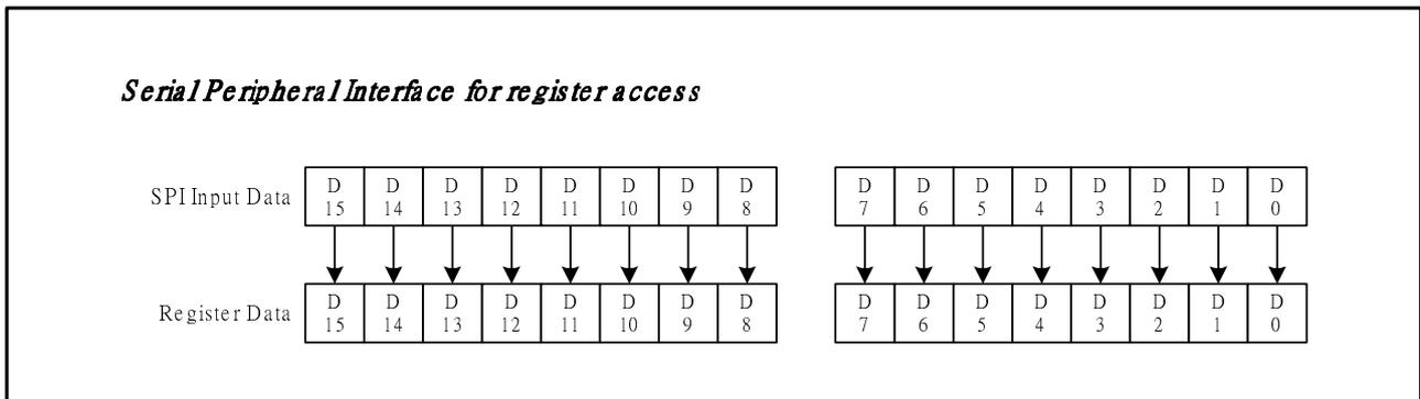
**Figure21 Register Setting with Serial Peripheral Interface (SPI)**
