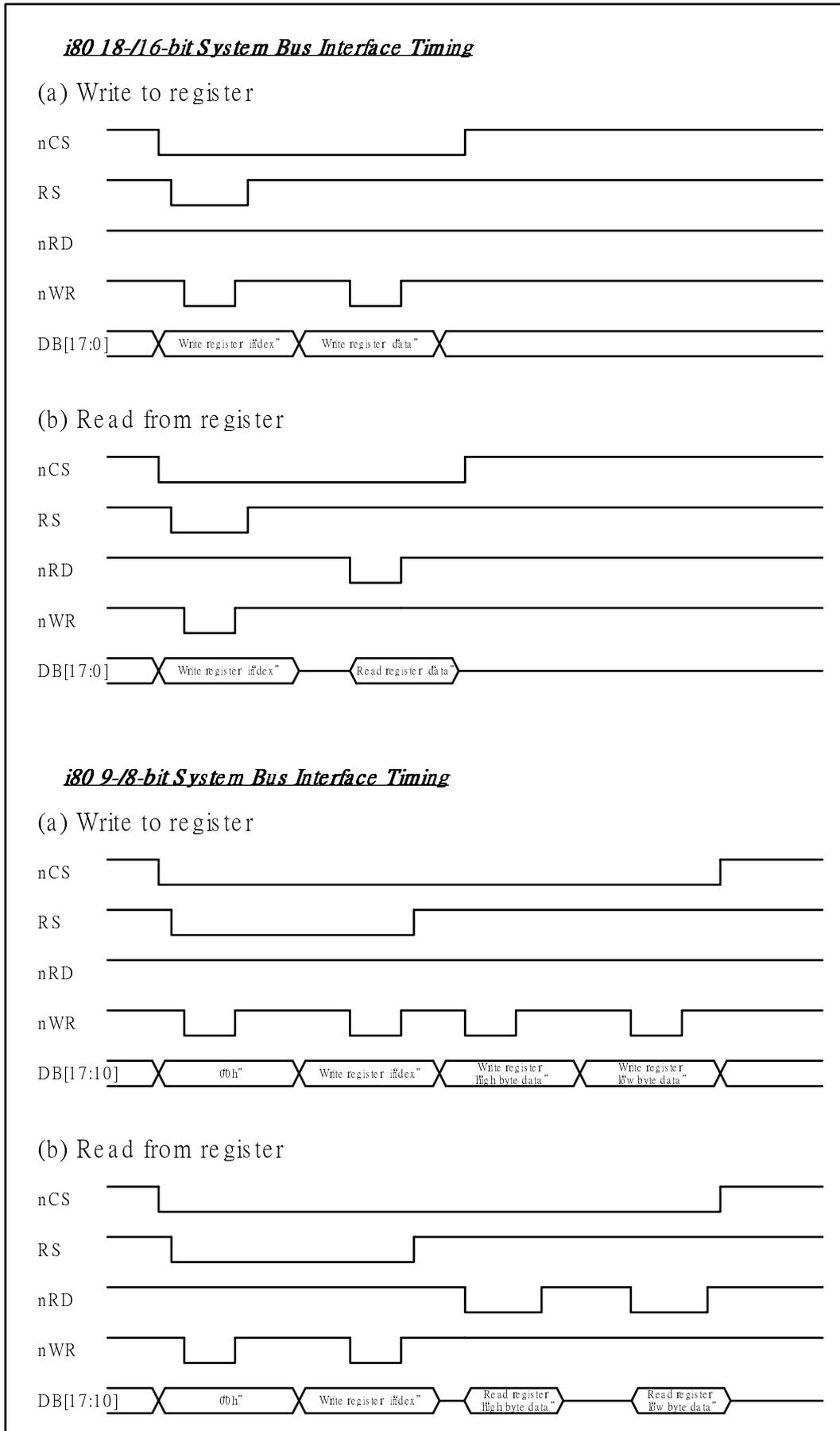
**Figure 23 Register Read/Write Timing of i80 System Interface**
