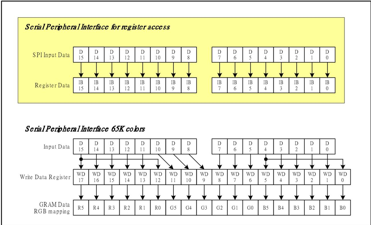
**Figure 6 Data Format of SPI Interface**
